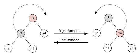
Figure 7.4: Tree left and right rotations
